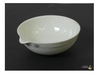
To heat liquids in the evaporating dish above a gas burner, use crucible tongs or place it on a tripod.
